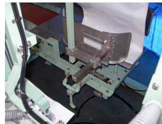
④ Bag holding carriage The filled bag is cradled during traverse for increased advance speed.
