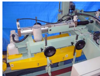
① Bag traverse cylinder Traverse cylinder is centered in order to reduce differential loading and vibration, resulting in increased capacity.
